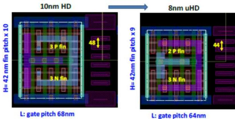
T18-4 Standard cell scaling from 10nm HD cell to 8nm uHD cell with gate pitch scaled from 68nm to 64nm, Mx from 48nm to 44nm with LE<sup>4</sup> process.
