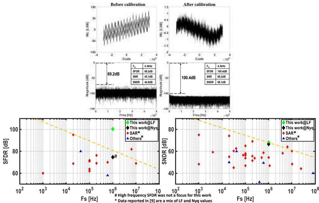
C9-1 >30dB linearity improvement (left-to-middle) from ADC background calibration along with state-of-art comparison graph (right).
