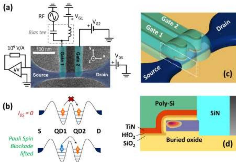
*T12-1* Schematic and top view SEM of the two-gate device with measurement setup description. Spin filtering mechanism across the double QD, (d) Cross-section along a gate and representation of the asymmetrical electron wavefunction along the mesa edge.
