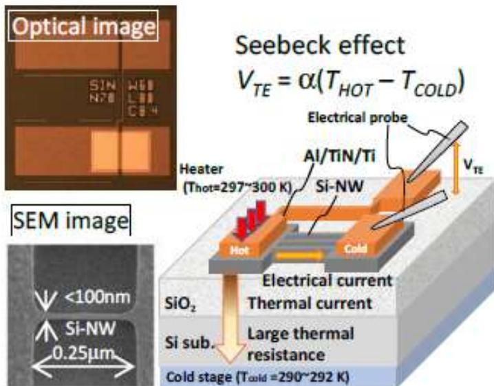
*T9-1 Fabrication of Si nanowire thermoelectric harvester where the Si nanowires were patterned using argon fluoride (ArF) immersion lithography.*
