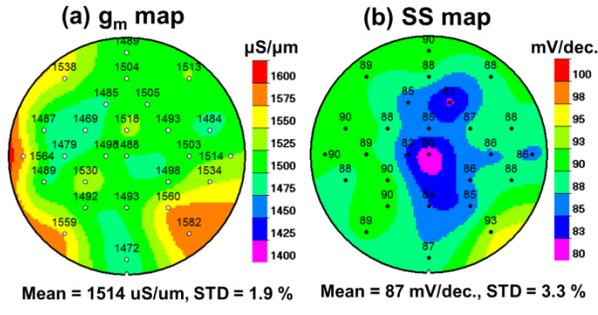
Fig. 9 The (a)  $g_m$  and (b) SS map across 300mm wafer, respectively. The good uniformity of  $L_g=120\text{nm}$  devices with high  $g_m$ (mean) of  $1514\ \mu\text{S}/\mu\text{m}$  (STD=1.9%) and low SS(mean) of  $87\ \text{mV}/\text{dec.}$  (STD=3.3%), respectively.
