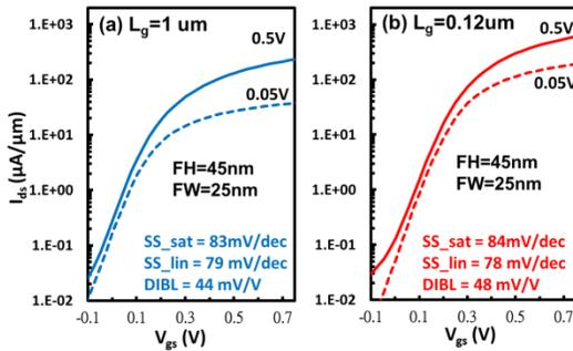
Fig. 4 Transfer characteristics of (a)  $L_g=1\mu\text{m}$  and (b)  $L_g=120\text{nm}$  devices with  $FW=25$  and  $FH=45\text{nm}$ .
