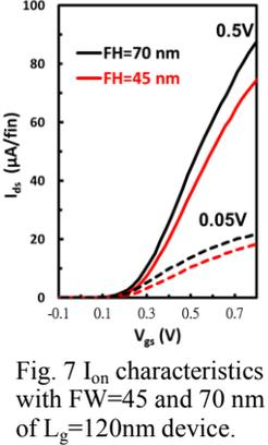
Fig. 7  $I_{on}$  characteristics with  $FW=45$  and  $70\text{nm}$  of  $L_g=120\text{nm}$  device.
