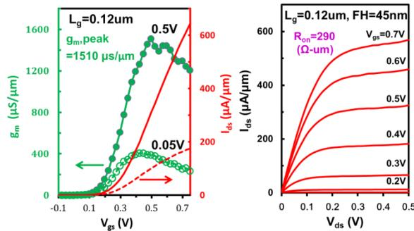
Fig. 5  $g_m$ - $I_{ds}$  and  $I_{ds}$ - $V_{gs}$  of  $L_g=120\text{nm}$  device at  $V_{ds}=0.5$  and  $0.05\text{V}$ , respectively.
