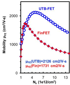
Fig. 13 Extracted field effect mobility ( $\mu_{FE}$ ) vs.  $N_e$  for UTB-, and Fin- FET.
