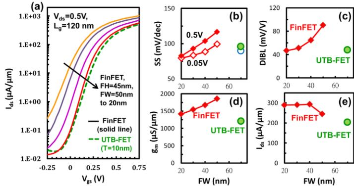
Fig. 3 (a)  $I_{ds}$ - $V_{gs}$  plot of UTB-FET ( $T=10\text{nm}$ ) and FinFET at  $V_{ds}=0.5\text{V}$ . (b) SS, (c) DIBL, (d)  $g_m$ , and (e)  $I_{ds}$  vs. FW for FinFET and UTB-FET.
