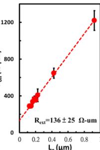
Fig. 10  $R_{on}$  vs.  $L_g$  of  $L_g=120\text{nm}$  device.
