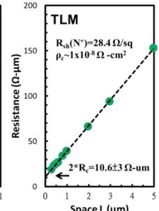
Fig. 11 TLM of metal-S/D junction.
