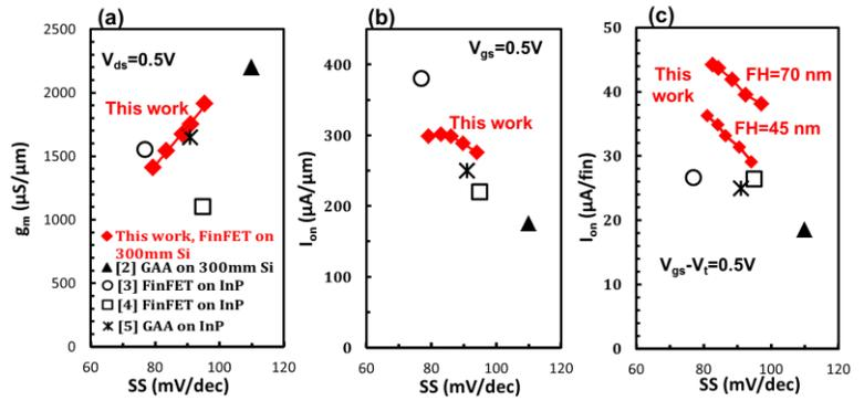
Fig. 14 Benchmarking of  $g_m$  (a) and  $I_{on}$  (b,c) vs. SS of  $\text{In}_{0.53}\text{Ga}_{0.47}\text{As}$  Fin- and nanowire- FET at  $V_{ds}=0.5\text{V}$  and  $V_{gs}=0.5\text{V}$  with  $I_{off}=100\text{nA}/\mu\text{m}$ . The  $g_m$  and  $I_{on}$  data are selected from device  $FW=20\text{-}50\text{nm}$ .
