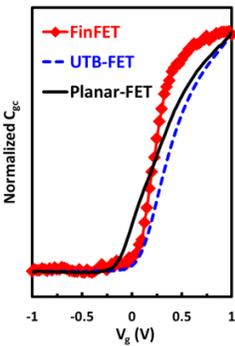
Fig. 12 Split C-V characteristics of planar- ( $T=50\text{nm}$ ), UTB- ( $T=10\text{nm}$ ), and Fin- ( $FW=25\text{nm}$ ) FET.
